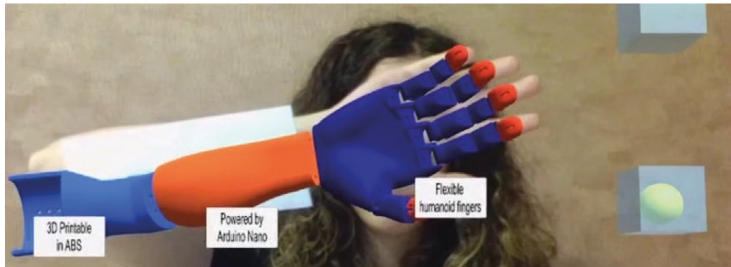
Fig. 3. AR exercise based on image tracking, developed in Unity and Vuforia. The target image is printed on a mobile card to simulate an arm prosthesis. When the user reaches the virtual ball, the prosthetic hand grabs it. Authors: G. Brero, A. Porcelli, M. Pettiti.
