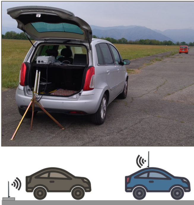
Figure 1: Test setup for measurements under NLOS conditions.
