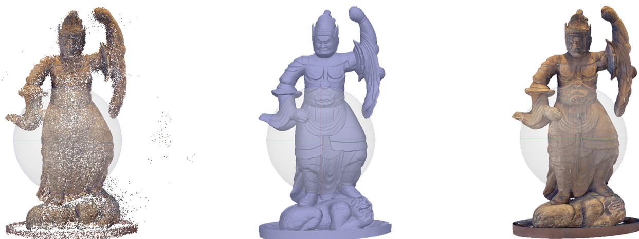
Figure 3. Creation of dense cloud, mesh model, textured model. Modelling: S. Tamantini.
