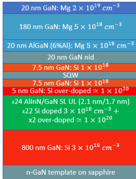
Figure 1: Diagram of the structure of the LED devices analyzed within this paper. Three identical wafers, differing only for the thickness of the quantum well, were fabricated. The properties of the quantum well are: indium content=20 %; thicknesses equal to 1.3 nm, 1.8 nm and 2.4 nm respectively for the wafers named A, B and C.
