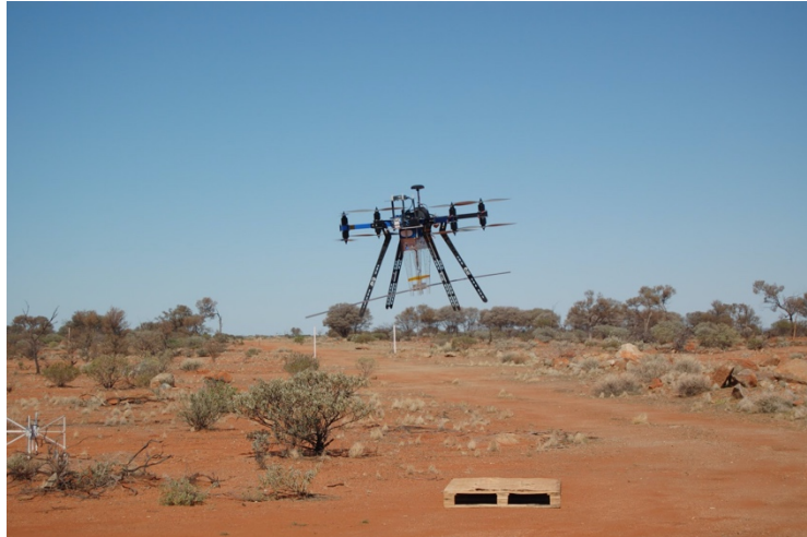
Figure 7: Octocopter used at MRO to characterize the station prototypes: the dipole antenna is visible.
