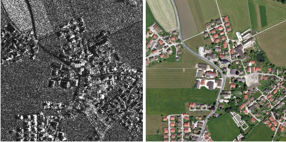
Fig. 1. Left: a single-look TerraSAR-X image acquired over Rosenheim (D). Right: an optical image of Rosenheim downloaded from Google-Earth Pro, co-registered with the SAR master. The noise intensity is extremely large for the SAR image, virtually zero for the optical image.
