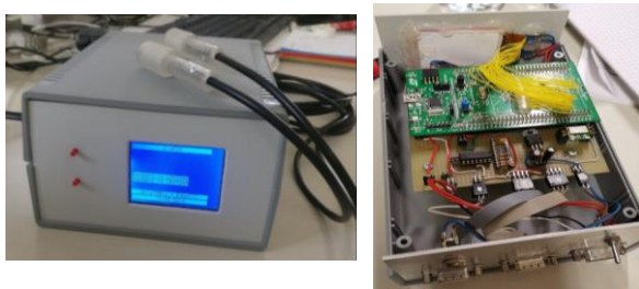
Fig. 2. Athos main device unit. On the left: the unit front panel, with the LCD (which shows the state of the sensors, their sample frequencies and the Bluetooth link state) and the button for the system reset. On the right: the internal interconnections between the STM32F429 Discovery Kit and the other system components.
