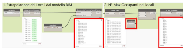
Figure 7. The script for the query focused on school strategic organization: Automatic selection of rooms of the school for calculation of the maximum capacity
