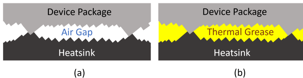
Figure 12 Heatsink-device mechanical coupling
