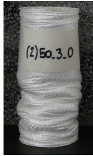
Figure 4: Final deformation of the specimen 50_3 under static axial crushing.
