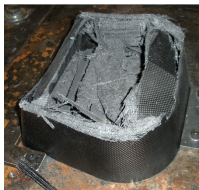
Figure 6: Deformation process of the CFRP impact attenuator: debris, bending and sharp break.
