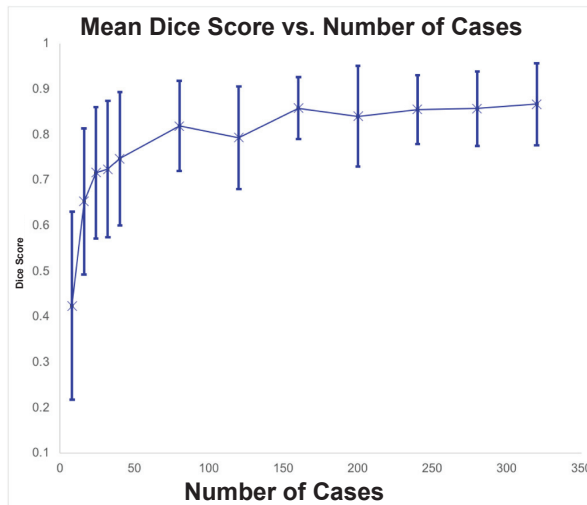
Figure 3. Dice score improved the most between 8 cases and 16 cases (0.424 to 0.653). The Dice score started to plateau after 160 cases which had a performance of 0.858. The Dice score only improved by 0.09 from 160 cases to 320 cases. The Dice score was plotted with error bars that show the standard deviation above and below that run’s mean Dice score. The standard deviation was lowest at 0.076 with 240 cases and highest at 0.206 with 8 cases.
