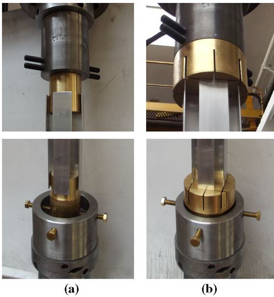
Fig. 11 Top and bottom end constraints for a free warping and b restrained warping
