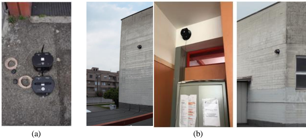
Figure 4. Sensing units with MEMS and FB accelerometers (a) and installation examples (b)
