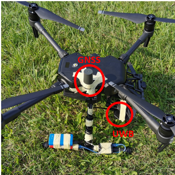
Figure 4. GNSS and UWB external sensors attached to DJI Matrice 210 drone.
