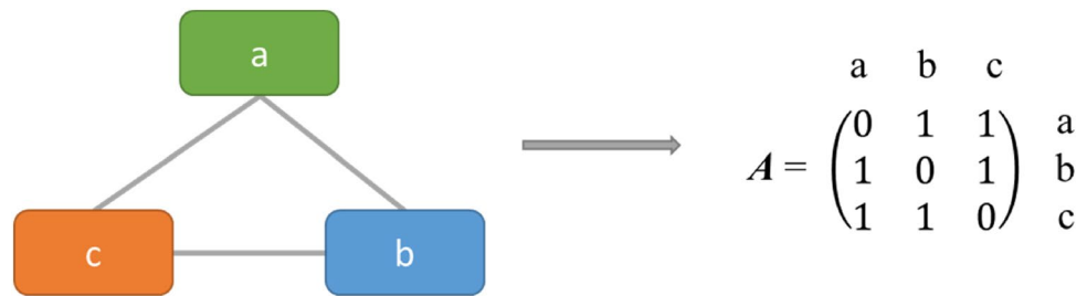
Fig. 1 Connectivity structure of a product composed of three parts and its associated adjacency matrix A
