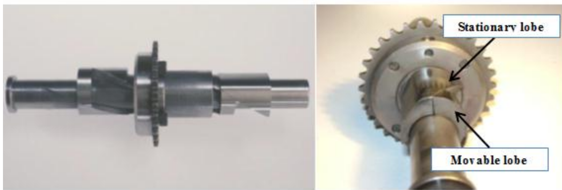
Figure 2.1. A prototype helical camshaft with the camshaft [1]
