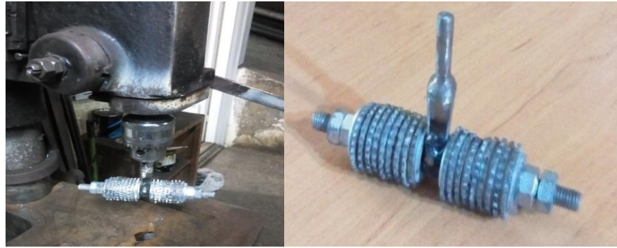
Figure 5. ASTM C944 chucked drill at the left and abrading cutter at the right.
