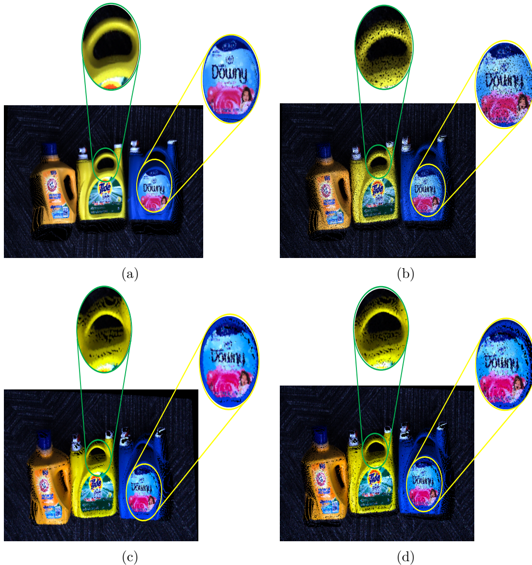
Figure 6.13: 3 Plastic Laundry Detergent on Carpet model: (a) ground-truth (b) noisy input, geometry denoised results by (c) proposed algorithm based on SGW using data-driven adaptive soft-thresholding (d) MSGW [17].
