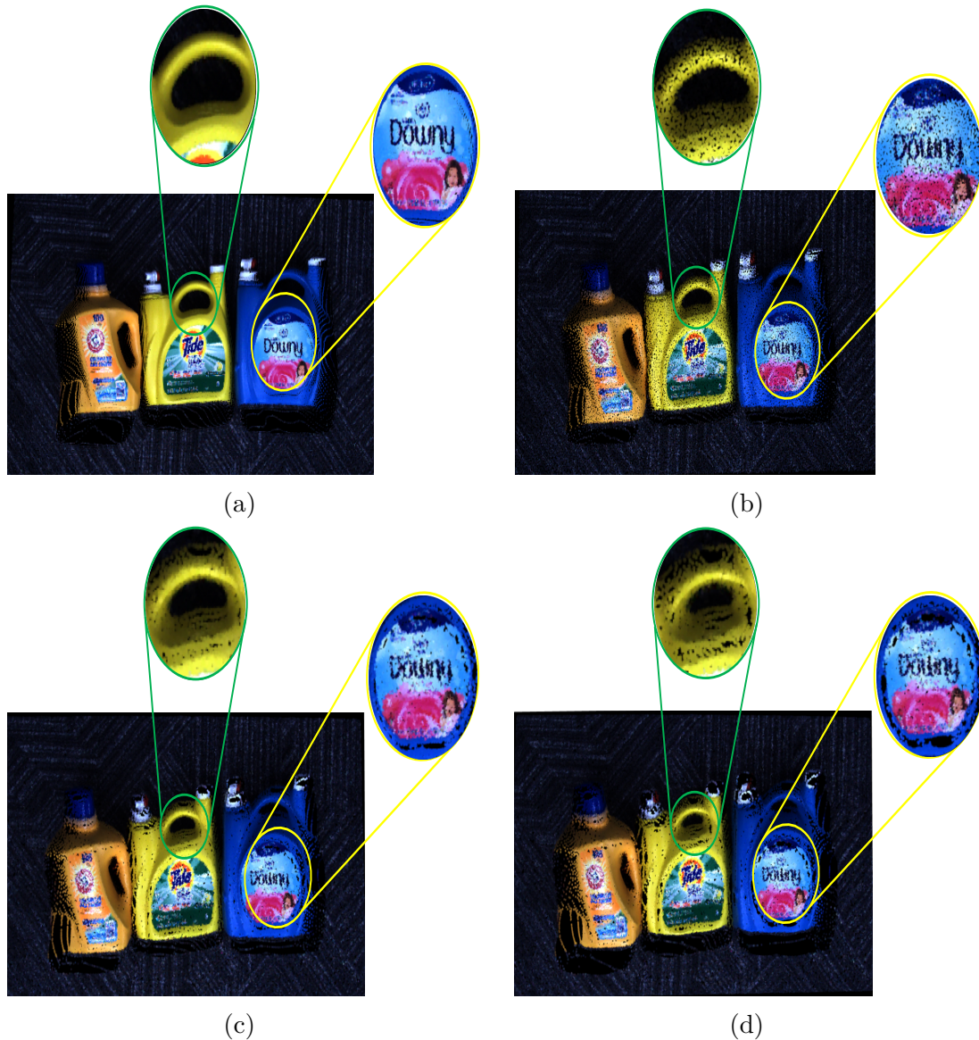
Figure 5.6: 3 Plastic Laundry Detergent on Carpet model: (a) ground-truth (b) noisy input, geometry denoised results by (c) proposed algorithm using Tikhonov regularization (d) geometry-only graph [112].
