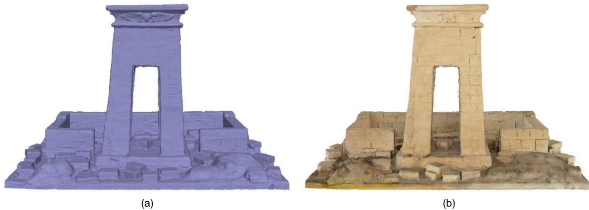
Figure 6: Photogrammetric outputs: a) 3D model of one of the modelled wooden maquettes (triangular mesh generated from the photogrammetric dense point cloud); and b) Photorealistic 3D model.
