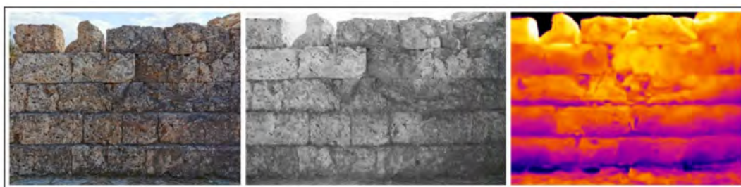
Figure 17. Reflectance images captured at the archaeological site of Lepreum: (from left to right) visible-spectrum, near-infrared, and a thermal-infrared image.
