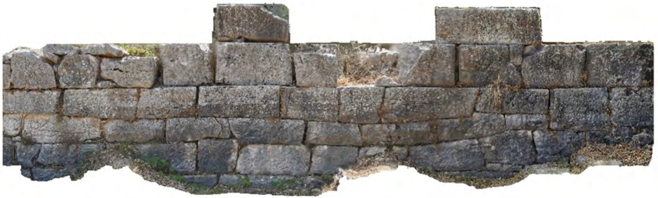
Figure 10. Orthoimage mosaic, cella wall remains at the Temple of Athena and Zeus Sotiros.
