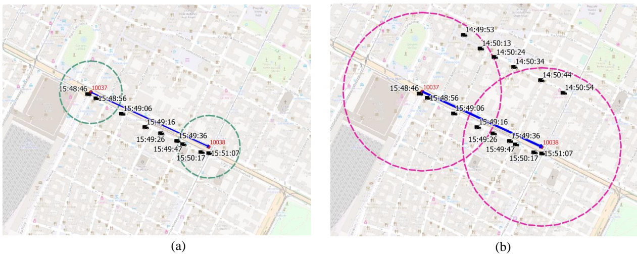
300 Fig. 6 Example of a link (blue line) connecting nodes 10037 and 10038, both representing intersections of two “Road2lanes” in the city centre. The 301 images represent two possible radii length: (a) 100 m and (b) 250 m (Source: QGIS).
