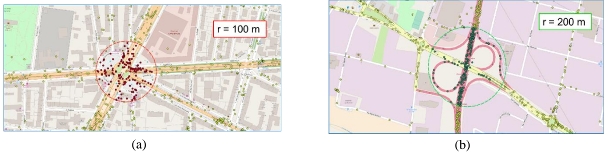
287 Fig. 5 Examples of the two classes of nodes and positioning data: (a) intersection connecting two “Road2lanes” and (b) a node at the crossing of a 288 “Motorway” and a “Road2lanes” (Source: QGIS).
