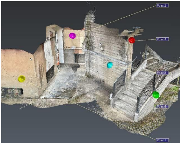
Figure 11. GCPs collimated in the point cloud (A) to evaluate the 3D accuracy on measured points.
