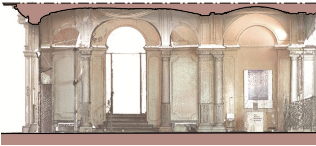
Figure 6. Longitudinal section at 1:50 scale of Palazzo Mazzonis atrium. Drawing: M. Vitali.
