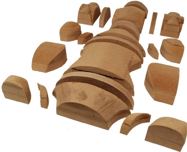
Figure 13. Wooden physical model aimed to tactile experience of the vault of Palazzo Mazzonis atrium. Digital prototyping: F. Ronco.
