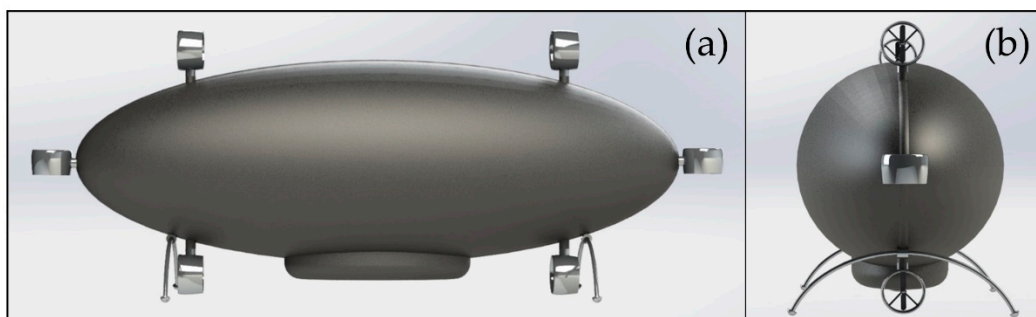
Figure 4. Conceptual sketch of the proposed LTA platform for land surveying. (a) Side view, (b) front view.
