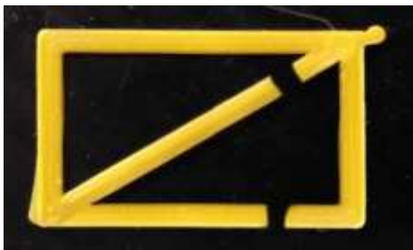
Figure 8. Printed sample with artificial defects.
