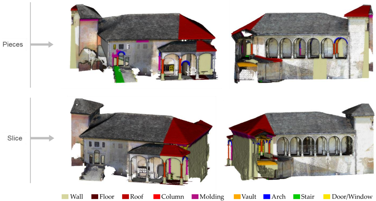
Figure 5. Subdivision of the test scene for the fine-tuning experiments. In the first case, only the coloured pieces have been used to fine-tune the network, while the RGB complementary part constitutes the test set. In the second case, an entire slice of the scene is used as input for the fine-tuning. The different colours correspond to the various classes.
