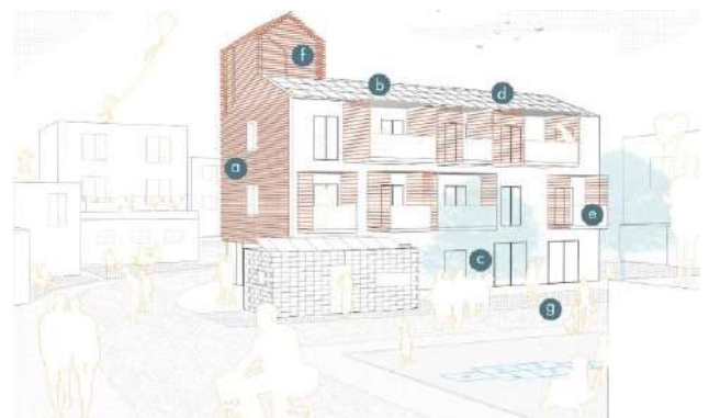
Fig.12: Design strategies. a. ventilated façade; b. photovoltaic modules; c. air to water heat pump; d. solar modules; e. shading system; f. solar chimney; g. rainwater reuse.
