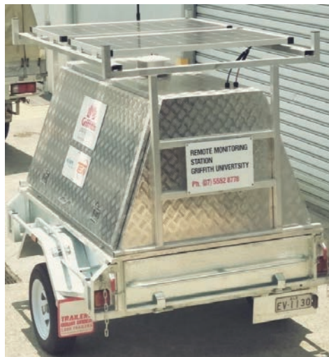
Figure 1. Trailer exterior modified with solar panels.
