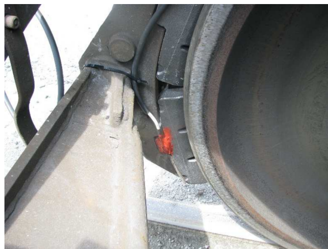
Figure 2. Brake block with temperature sensor.
