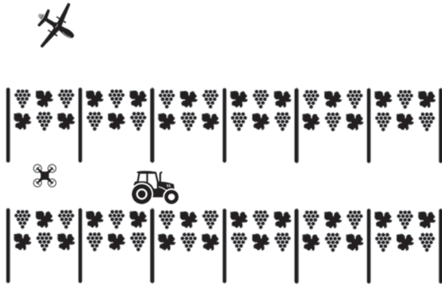
Fig. 1. Collaborative fleet composed by a FW-UAV for remote sensing task and UGVs and RW-UAVs for spraying and shredding operations in sloped vineyards.
