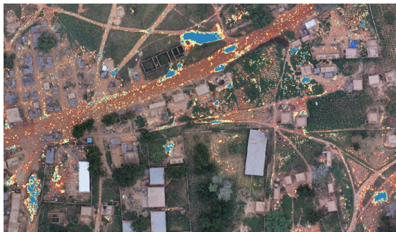
Figure 88. Detail of the depressions identified through the DTM analysis in Larba Birno. The small and shallow depressions are DTM artifacts created by the roughness of the soil. Some depressions are well defined (blue spots), while others are noisy due to irregularities on the ground due to mud and water.
