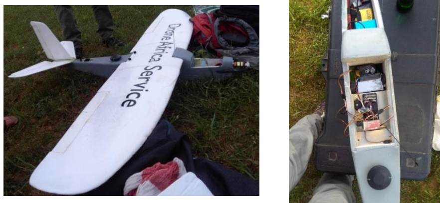
Figure 78. Left: UAV system built by Drone Africa Service. Right: Detail of the UAV body. It is visible that the Raspberry Pi sensor is mounted on the UAV system. 3.5 inches screen and the GPS receiver.
