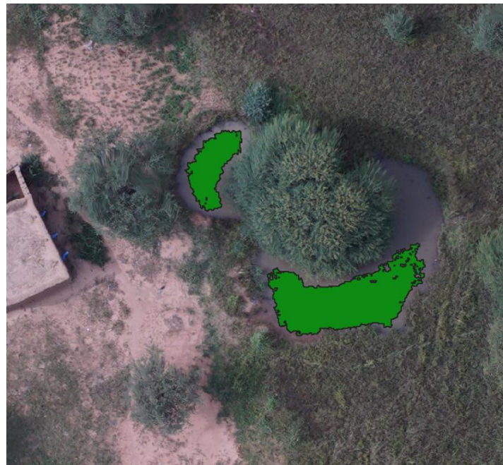
Figure 92. TSWB detected by NDWI analysis (green features) and partially developed under a tree crown. It was not detected by the DTM method.
