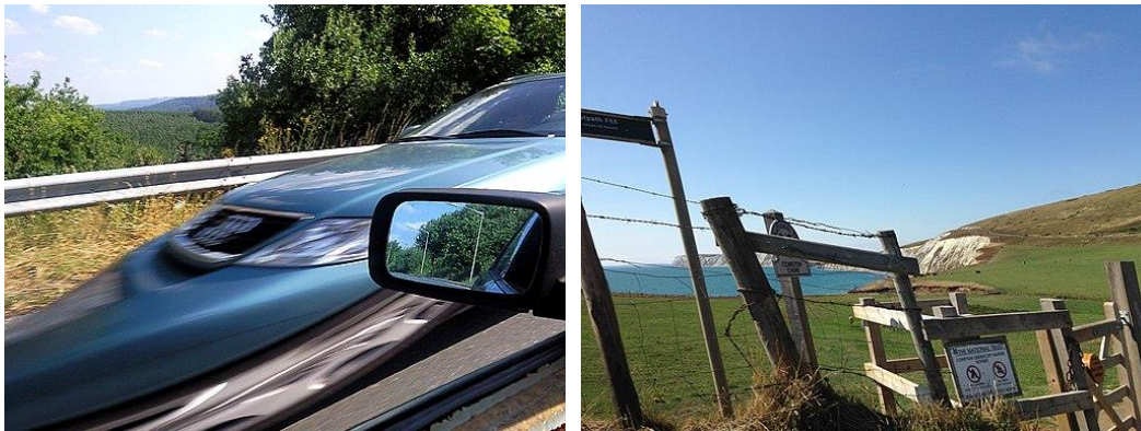
Figure 5. Two widespread effects of rolling shutter sensors. An example of the distortions caused by the rolling shutter of a fast-moving object (car) is on the left. On the right, the distortion caused by the rolling shutter is used for capturing an image of a static scene (fence) from a moving means. CC BY-SA 4.0 via wikimedia.
