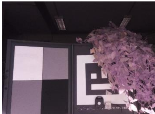
Figure 56. Picture of the calibration scene taken by the NoIR camera. On the left, the calibration target comprises four panels (white, light grey, dark grey, and black). On the right side of the picture, a plant. At the bottom of the picture is visible, the irradiance sensor of the hyperspectral.
