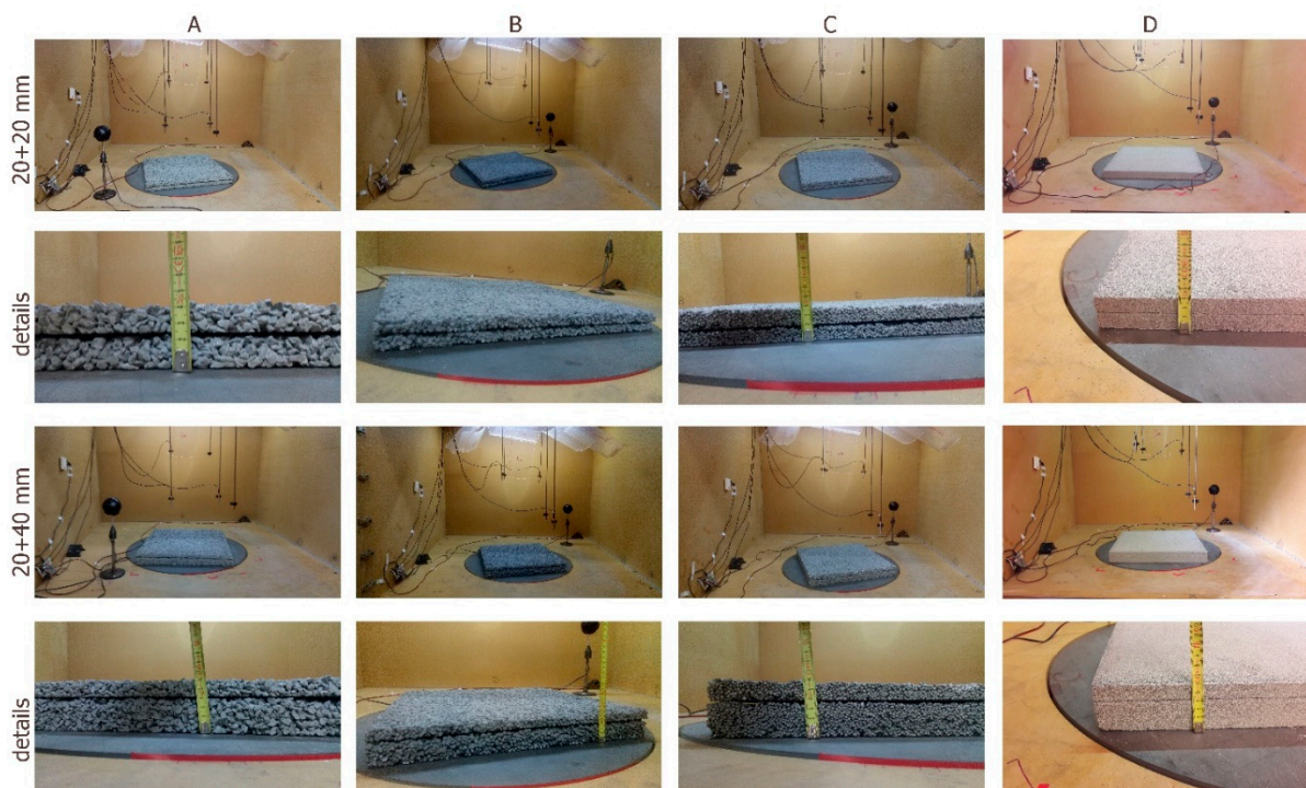
Figure 2. Multiple layers of 20 + 20 mm and 20 + 40 mm. Sample (A): crushed normal weight aggregates 4–8 mm; Sample (B): round lightweight aggregates 4–8 mm; Sample (C): round lightweight aggregates 2–4 mm; Sample (D): round lightweight aggregates 0.5–1 mm.
