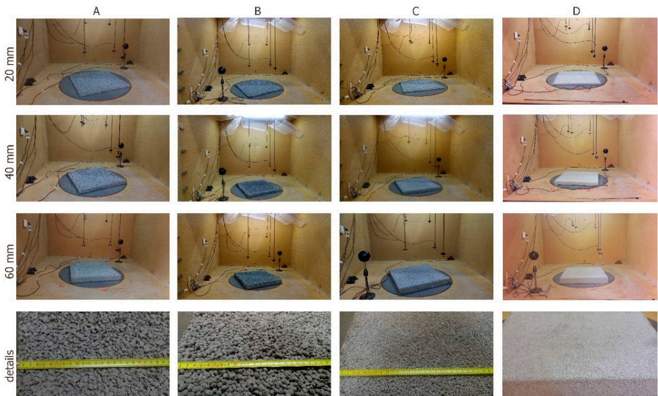
Figure 1. Sample (A): crushed normal weight aggregates 4–8 mm; Sample (B): round lightweight aggregates 4–8 mm; Sample (C): round lightweight aggregates 2–4 mm; Sample (D): round lightweight aggregates 0.5–1 mm.
