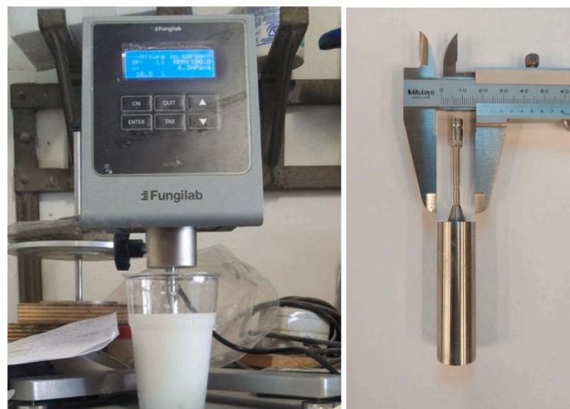
Fig. 3. Rotational viscometer used (on the left) and spindle used (on the right). Spindle not to scale.
