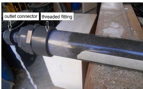
Fig. 6. Details of the sample tail. Left: photograph during the grouting phase. Right: a simple scheme (not to scale) of the filter system.
