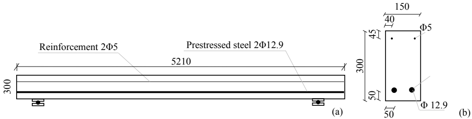
Figure 2. Geometrical features of the beams [in mm]: (a) Longitudinal view and (b) Transversal cross-section.
