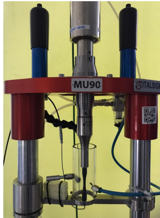
Figure 1. Ultrasonic fatigue testing machine MU90.
