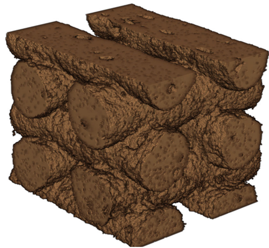
Fig. 3 3D geometric model based on \mu - CT scans of the printed scaffold
