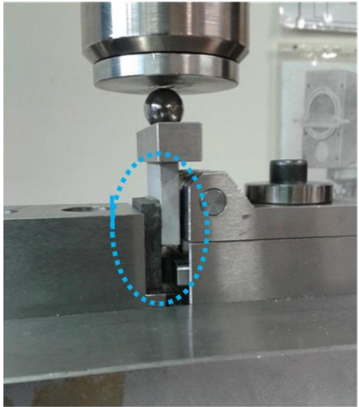
Figure 3 Test configuration and geometry of a joined specimen for the single lap offset test under compression.
