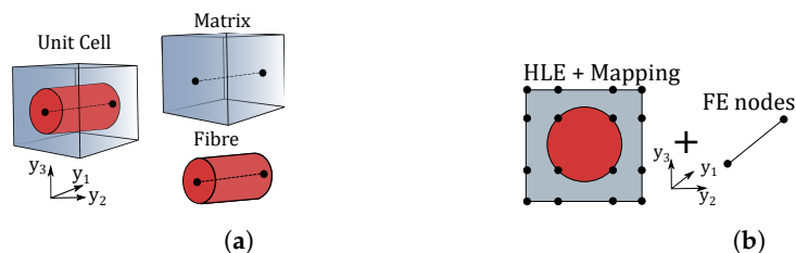
Figure 5. (a) Component-wise modelling of composite microstructure with different phases. (b) Kinematics used to define the RUC cross-section.
