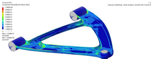
Figure 31. Contour plot of composite ply failure: braking load case (shuffle optimization)
