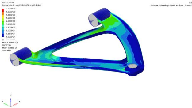
Figure 33. Contour plot of composite strength ratio: braking load case (shuffle optimization)
