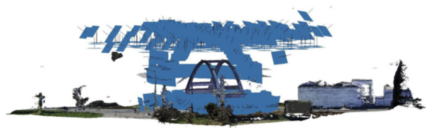
Figure 6: Image alignment and tie points generation.
