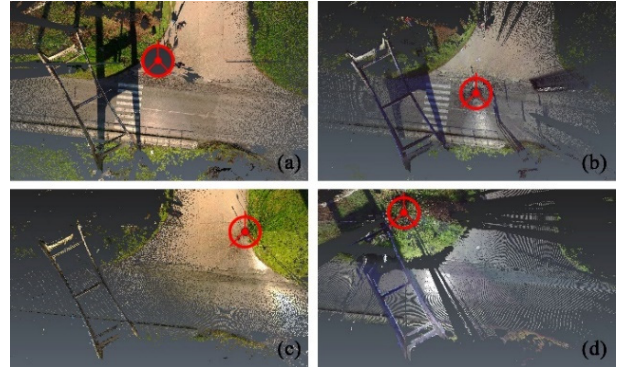
Figure 9: Acquisition scheme of each of the considered LiDAR scan (the position of the laser scanner is indicated by the red symbol): a) scanner on the pneumatic telescopic pole, acquisition from medium distance; b) scanner on ground level, acquisition from medium distance; c) scanner on ground level, acquisition from long distance; d) scanner on ground level, acquisition from short distance.
