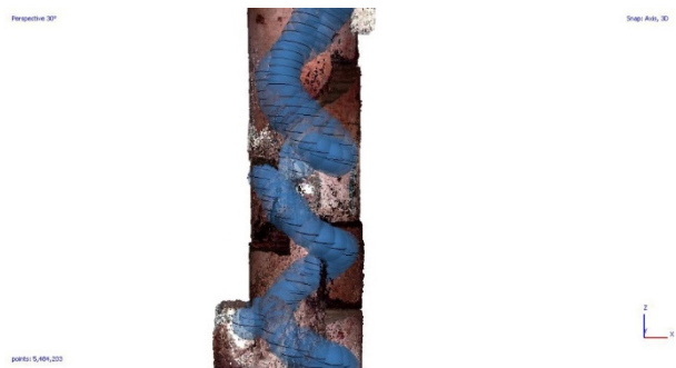
Figure 10: Extract of the acquisition geometry of the 360° dataset (blue spheres represent camera position, black letters are the name of the single images).
