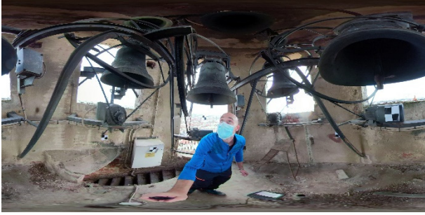
Figure 7: Example of spherical images (equirectangular projection) acquired in the bell tower with the GoPro Fusion.
