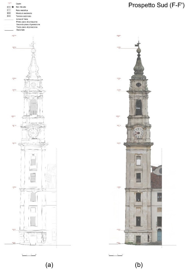
Figure 13: Example of one of the 2D architectural drawing (south facade): a) based on the 3D integrated survey; b) overlaid with the orthoimage.
