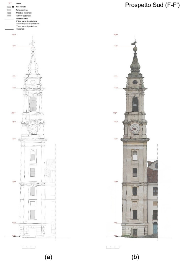
Figure 13: Example of one of the 2D architectural drawing (south facade): a) based on the 3D integrated survey; b) overlaid with the orthoimage.
