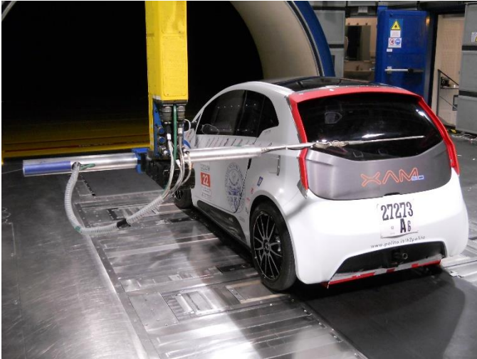
Figure 5 - Pressure field measurement with 14-holes probe
