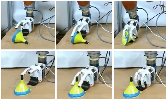
Fig. 5: Experiment 1: grasp success (top) and failure (bottom) of the funnel.
