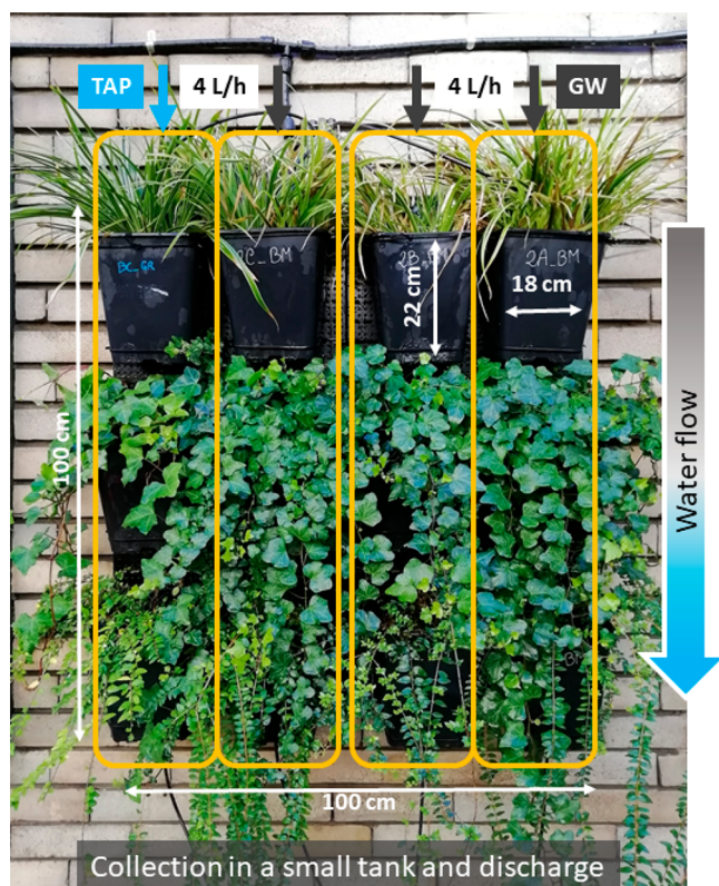
Figure 1. Modular panel of the green wall. All columns (marked in yellow) were identical except for the type of irrigation, and each worked independently. Three columns of this panel were fed with graywater (GW), and one was fed with tap water (TAP).
