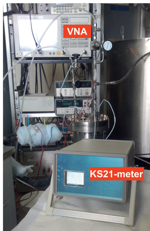
(b) Read-out systems: laboratory VNA vs. developed low-cost KS_{21} -meter.
