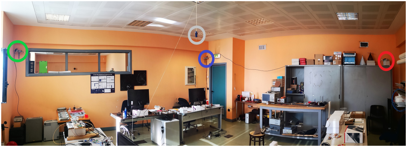
Fig. 16. Indoor laboratory measurement setup. In green, red, blue and gray are highlighted respectively the three sensors and reference tag positions.
