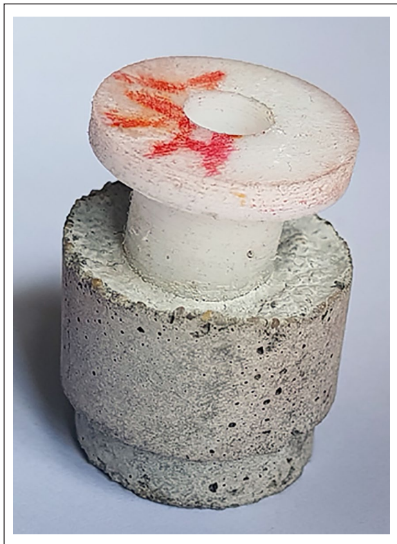
Figure 2. Mortar sample with an internal embedded pH sensor at the bottom of the Teflon piece which hosts the optical fiber.
