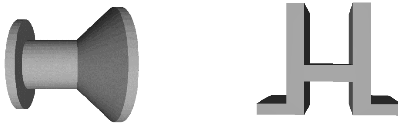
Figure 3 - Prototypes of a connector for a pump and of a door's hinge
