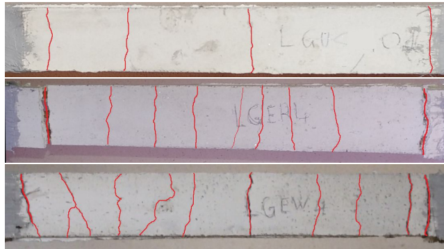
Figure 15: Near failure crack pattern in G-UC (top), G-ER (middle) and G-EW (bottom) specimens
