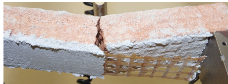
Figure 8: Typical delamination failure mode for brick bending in the G-ER and G-EW groups
