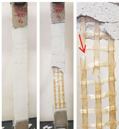
(a) Fabric failure
